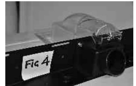
• Insert the Csk head screws through the two Csk Ø6mm holes in the vertical face of the Metal Fence, allowing the heads to lie 'flush' with the fence surface.
